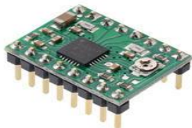
Fig. 11: A4988 stepper motor driver
